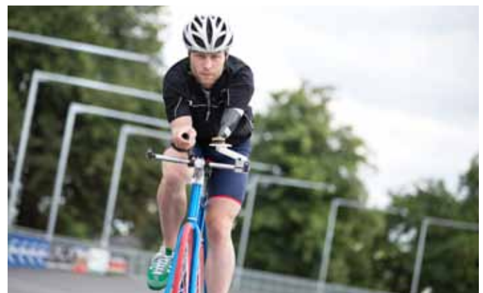
Handlebar attachment to enable standing starts for Paralympic cyclists
