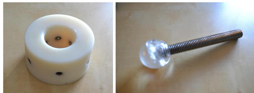
Figure 6 The new attachment method of the prosthesis to the prototype. The core (right) is supposed to be embedded in the prosthesis and the shell (left) is bolted with a countersunk screw at the top of the top nylon piece. The sphere of the core has indents around it for the spring plungers in the shell to hold it in place.
